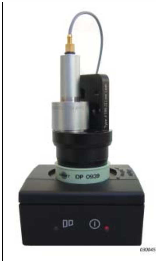
Fig. 2 The coupler mounted with the Standard Adaptor Ring for on-the-line sensitivity verification with Sound Level Calibrator Type 4231 and Calibration Adaptor DP 0939
